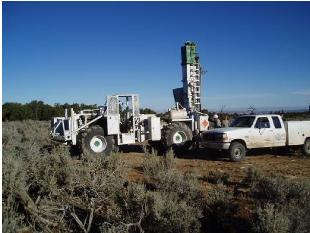
Picture C-3: Buggy-drill with drill mast raised into drilling position.
