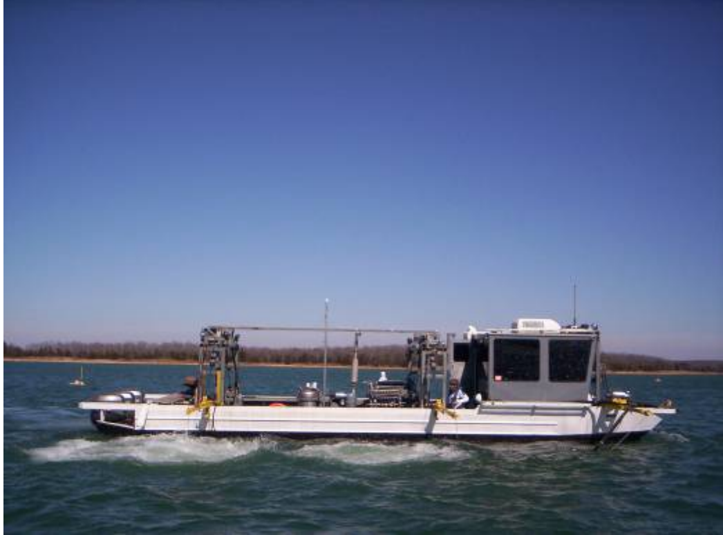
Picture C-9: Effects on water surface from firing the air-gun array.
