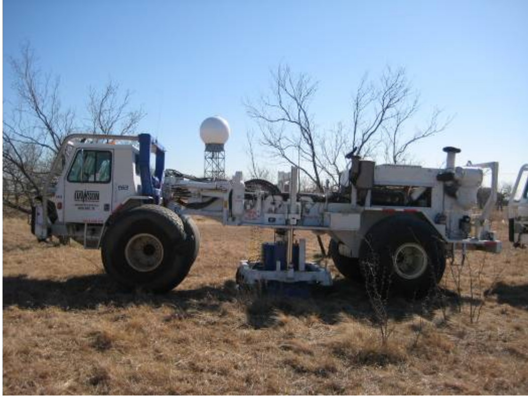
Picture C-1: Vibroseis buggy (buggy-vibe) with plunger/plate lowered into "shake" position.
