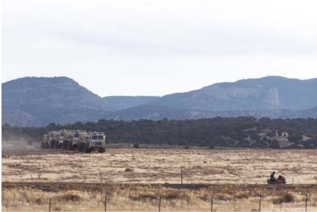
Picture C-2: A line of four buggy-vibes moving between source points.
