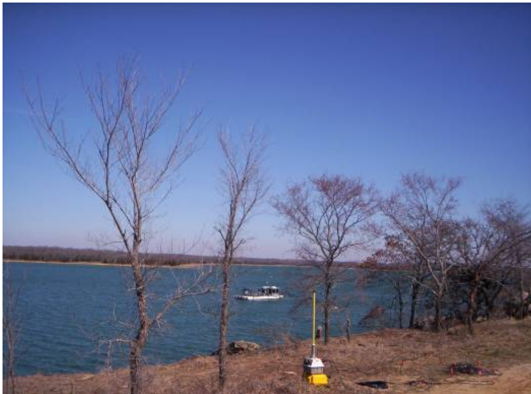
Picture C-10: Air-gun boat crossing a connected submerged and on-land receiver line during operations.
