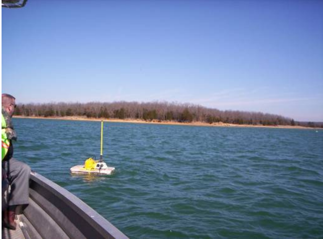
Picture C-11: Buoy mounted with recording equipment, batteries, and antenna plus cable connection.
