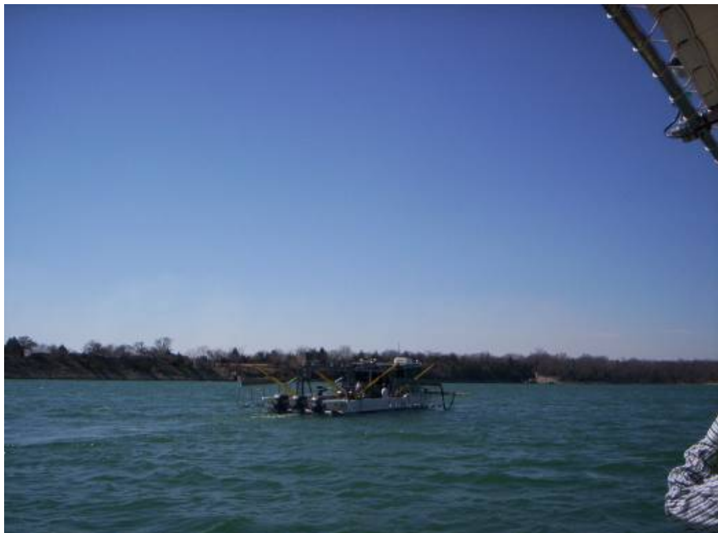
Picture C-8: Air-gun boat with air guns suspended above the water surface.
