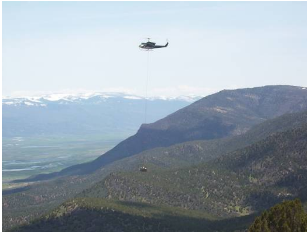
Picture C-5: Heliportable drilling equipment being moved by helicopter.
